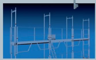
The safety guardrail remains in the scaffold permanently.
